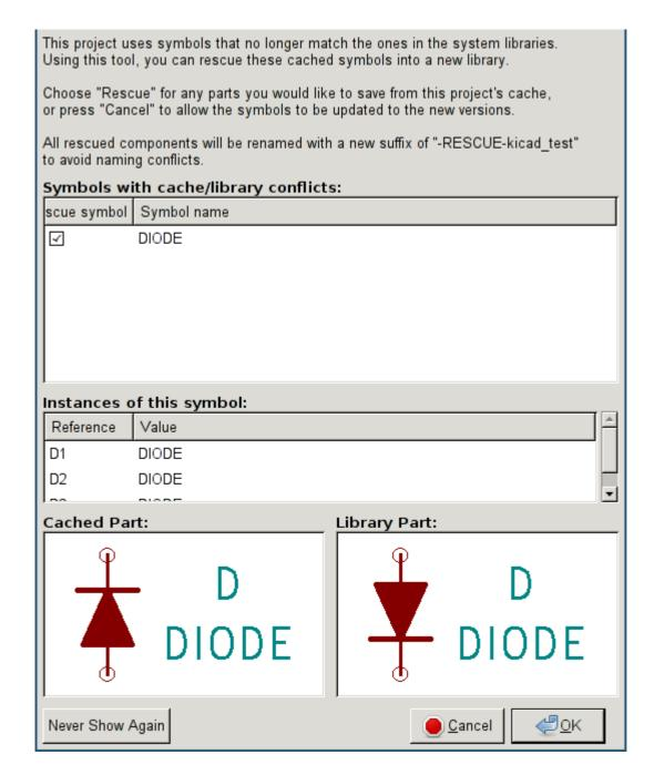
You can see in this example that the project originally used a diode with the cathode facing up, but the library now contains one with the cathode facing down. This change would break the schematic! Pressing OK here will cause the symbol cache library to be saved into a special rescue library and all the symbols are renamed to avoid naming conflicts.
