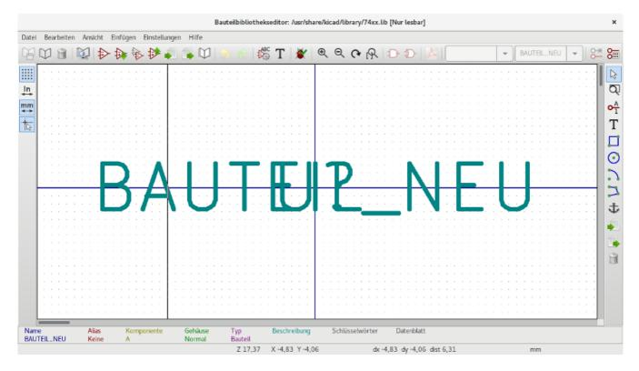
The blue cross in the center is the symbol anchor, which specifies the symbol origin i.e. the coordinates (0, 0). The anchor can be repositioned by selecting the \* icon and clicking on the new desired anchor position.
